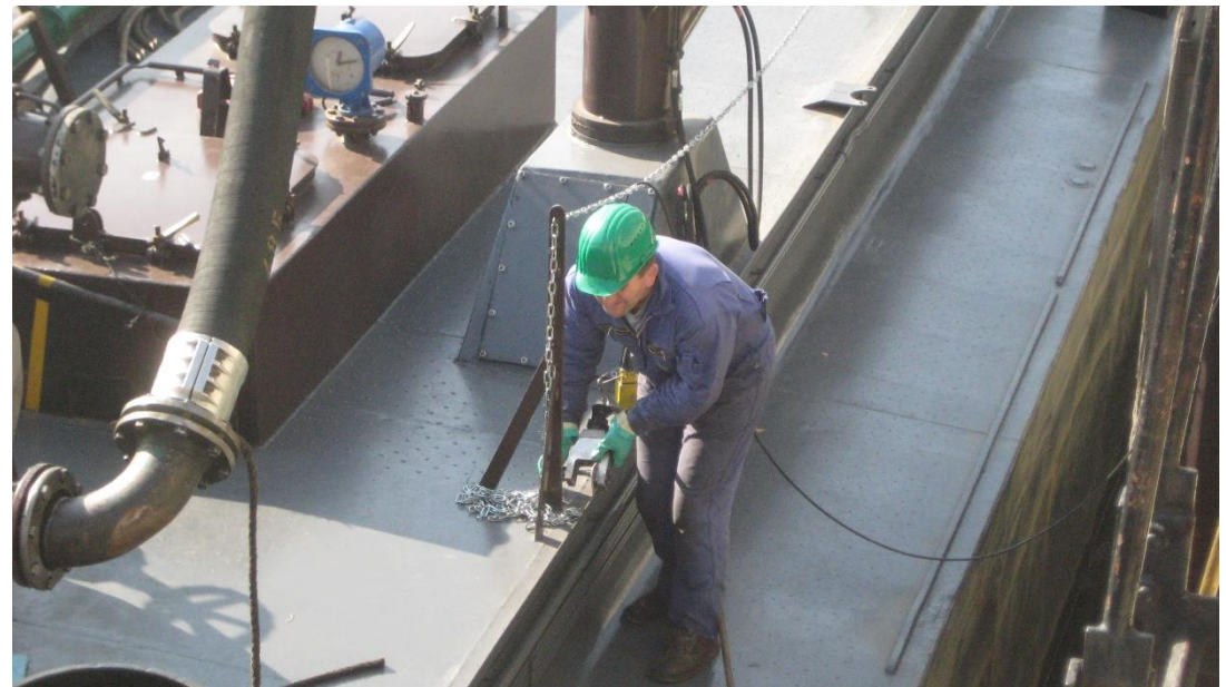
Attaching Grounding Clamp to Ship
